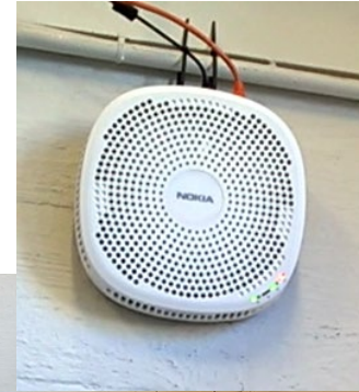
Indoor LTE/Wi-Fi picocell for wireless communication
