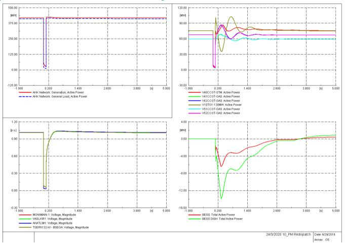
24/03/2020 22:00 Scenario A3. Load 416.9MW. RES 0% Re-dispatch: V50CCGT-STEAM off. V1STG-130MW on
