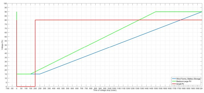
> Fault ride-through capability does not mean that plant can remain connected under any voltage drop/duration
