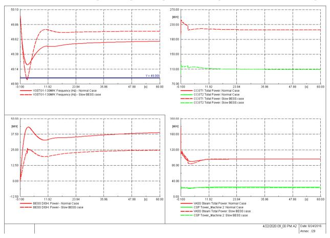
22/04/2020 21:00, Scenario A2. Total Load: 510,5MW. Loss of 88.1MW (17,2%)
