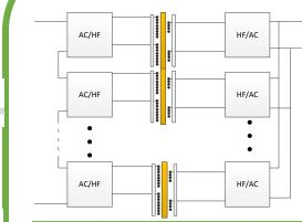
Innovative SST module based on a bidirectional IPT static system
