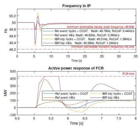
Fig. 5. Frequency in IP after reference incident and IBR trip, FCR in IP provided either by conventional technologies orHEs
